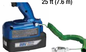
Attach cup with solvent, set to "Clean" and run upside down.
