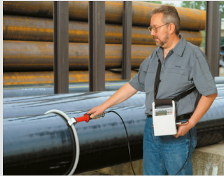
Porosity detection on pipelines
