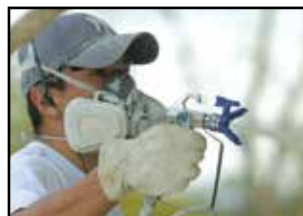
FTx 4-finger gun trigger – full length trigger is easier to hold in continuous spray.
