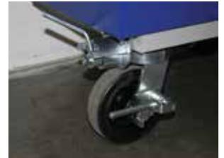
Rear Wheel System with release and brake.
