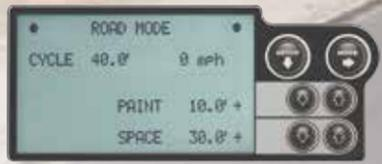
**Auto-Layout System** New automatic gun system allows marking to be done with guns rather than with the assistance of aerosol cans.
